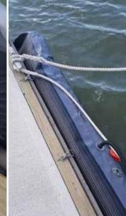
Fixing points. 3000 mm Protector fenders have 5 x fixing points (2 x being spare).
