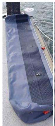
Unpack Fender. Lay fender flat, D - Ring side up with rings facing towards the boat.
